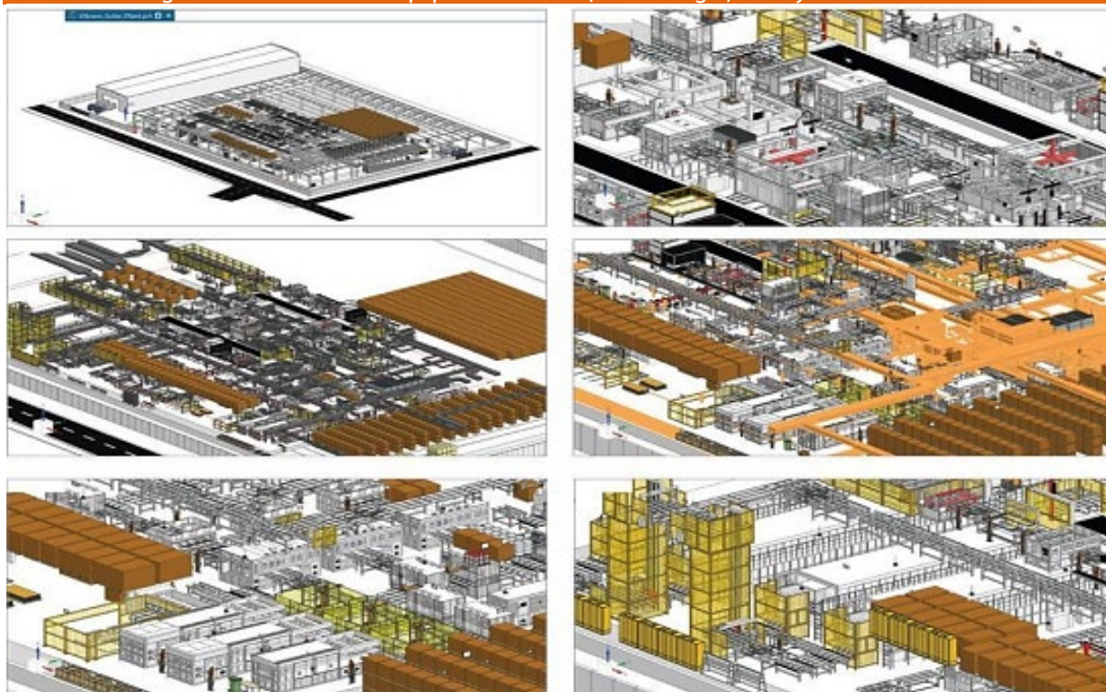
Exhibit 4: 3D digital twin model of all equipment in Falta (West Bengal) facility
